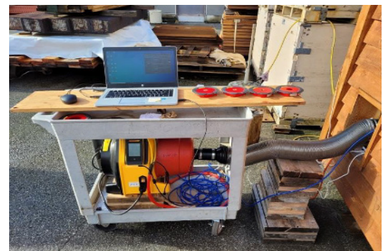
Figure 5. The blower used for creating a pressure difference between the inside and outside of the RAIN chamber (source: FPInnovations).
